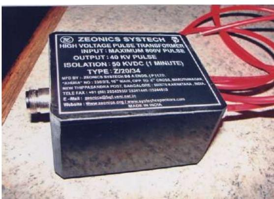
Input Voltage : 800V to 900V; pulse 1 $\mu$ s to 5 $\mu$ s
