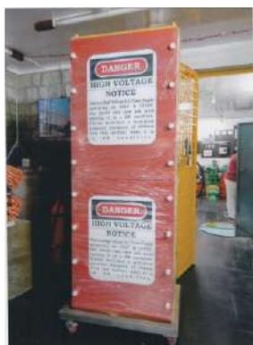
The entire rack is isolated to take a floating HV power supply of 150kV DC
