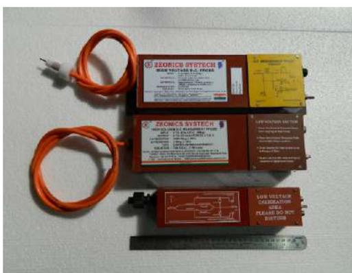
Working Voltage : 50kV / 60kV / 100kV DC
