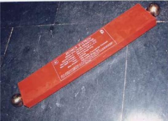
Working voltage : 200kV AC; maximum 300kV AC
