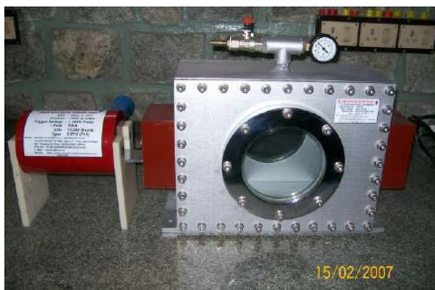
Input : DC of 20kV to 50kV DC stored energy of 1kJ to 5kJ
