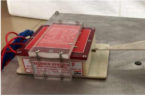
Voltage : 25kV/50kV/Output
