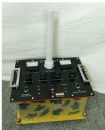
A pre-ionized gas-based E-field system which can detect electric fields which can occur in the atmosphere.
