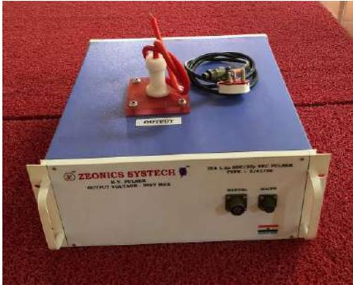
Pulse : 1.2/50 $\mu$ s at 25kV output
