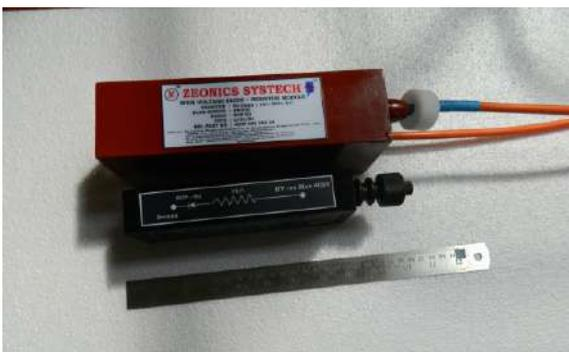
Working Voltage : 50kV DC  $\pm$  1%
