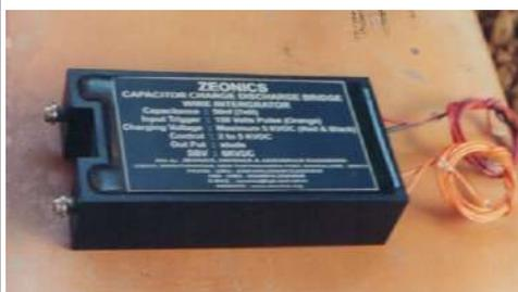
Input voltage : 3kV DC
