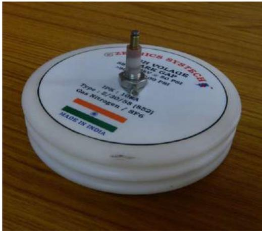
SBV : 60kV at 50psi, > 90kV at 100 psi,  $\approx$ 120kV
